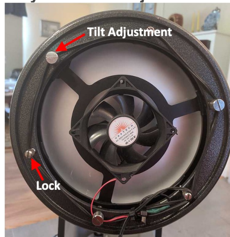
Figure 12: Primary Mirror Tilt Adjustment and Lock Screws
